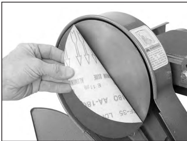
Figure 30. Installing sanding disc onto cast iron plate.
